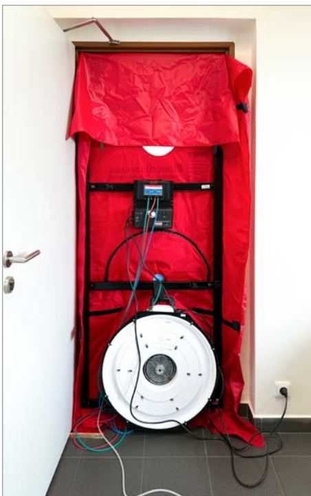
To verify the airtightness of the building, we perform tests using a professional Blower Door test measuring system
